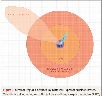
The relative sizes of regions affected by a radiologic exposure device (RED), a radiologic dispersion device (RDD), an improvised nuclear device (IND), and a sophisticated nuclear weapon are shown. The fallout zone shown is for the IND.
